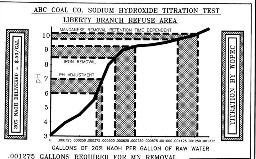
.001275 GALLONS REQUIRED FOR MN REMOVAL \$.000638/GALLON OF RAW WATER FOR MN REMOVAL AVERAGE FLOW RATE = 175 GALLONS PER MINUTE ANNUAL COST = \$ 58,683.00
